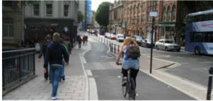
Fully kerbed segregated cycle track
