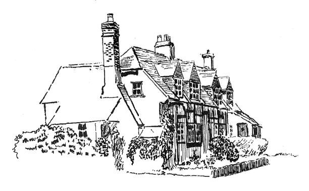
**Roof Detail** - The early roofs are generally of red/orange clay plain tiles with gabled, hipped or half-hipped varieties. Some thatch roofs are also evident as well as slate.
