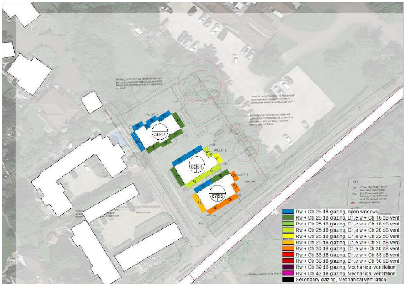
Figure 4: Glazing and ventilation strategy – First Floor
