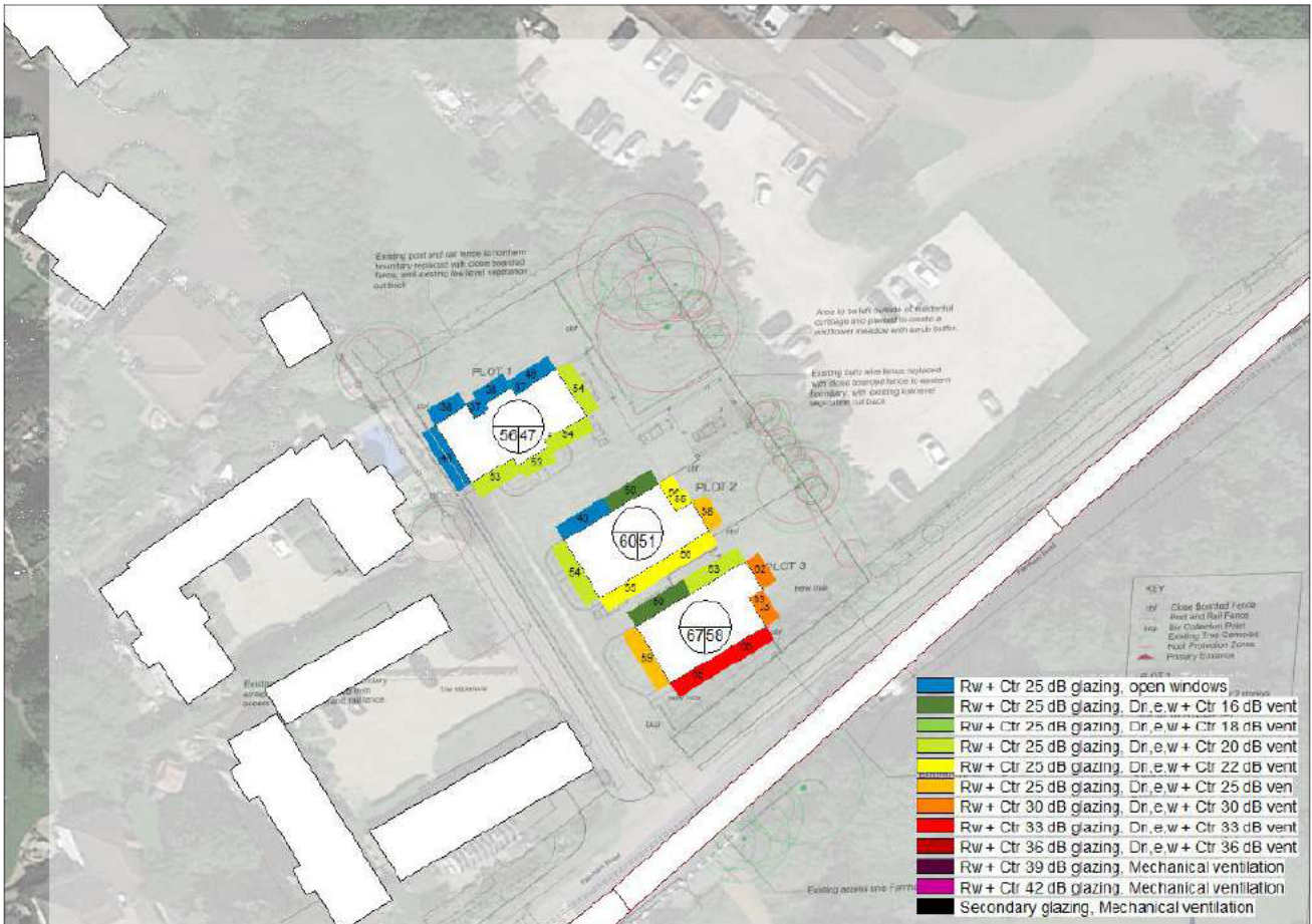
Figure 3: Glazing and ventilation strategy – Ground Floor
